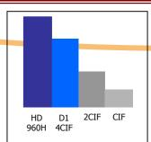
This comparison demonstrates the differences in recorded picture quality. The height of each is effectively comparing the number of pixels.
